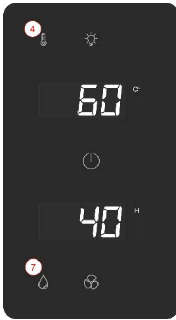
Fig. 12 Switching on the “Finnish sauna” or “Steam sauna” operating mode
